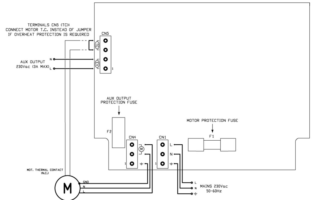
Pic.1 Wiring diagram
